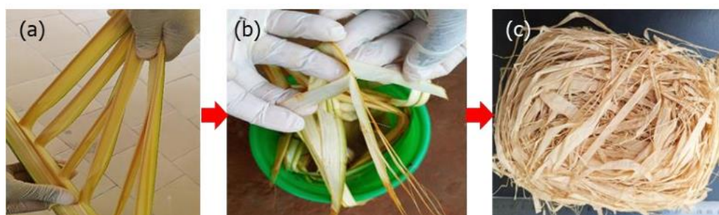
Fig. 1. Extraction process of Raffia leaf cuticles: (a) stripping the Raffia spear; (b) manual peeling of the cuticles after 14 days of retting in fresh water; (c) extracted fibrous cuticles.
