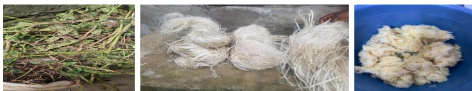
Figure 1 — (a) Raw okra stems; (b) fibers after extraction and washing; (c) fibers after alkaline treatment and bleaching
