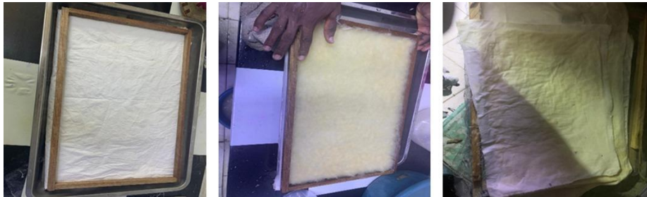
Figure 2 — Wallpaper fabrication process: (a) mold preparation; (b) pulp forming; (c) drying
