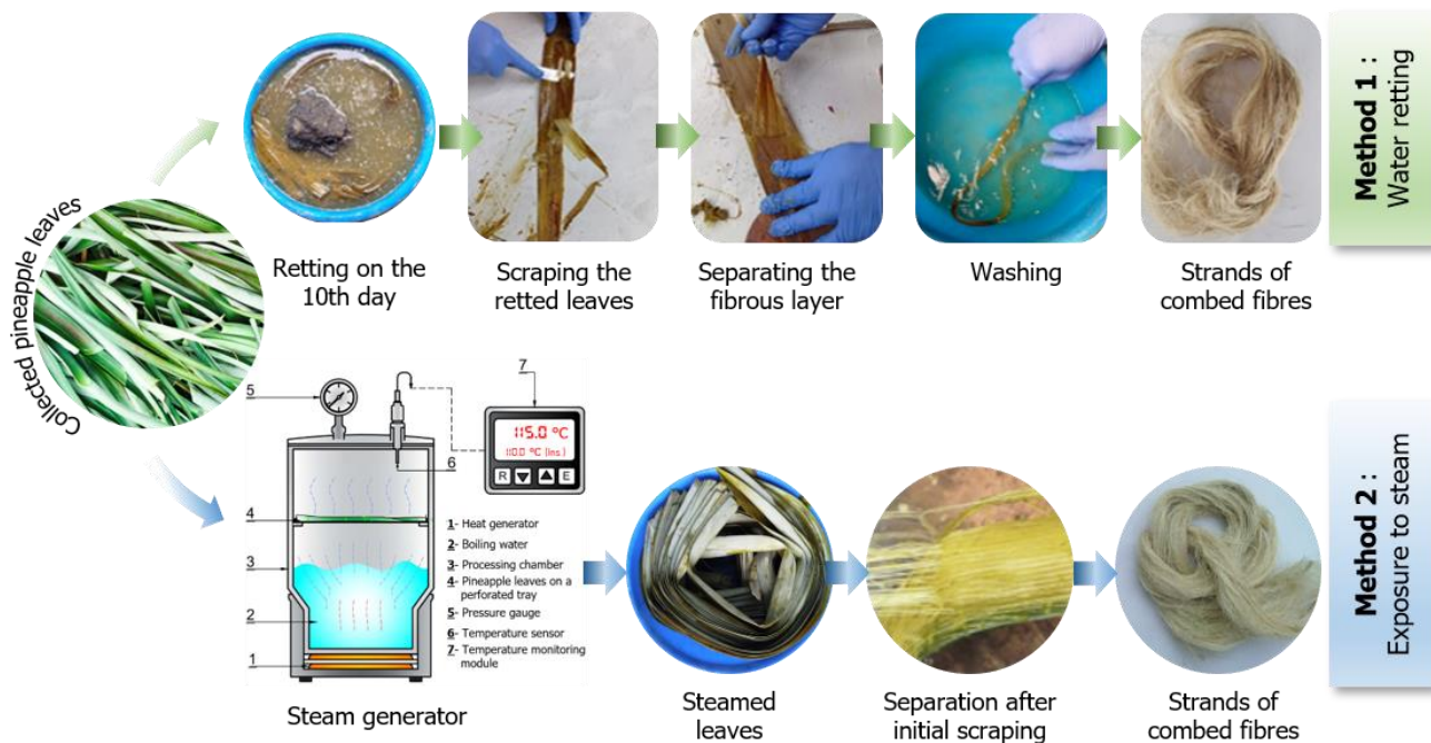
Fig. 1. The process of extracting fibre strands by water retting (top) and steam treatment (bottom) of pineapple leaves
